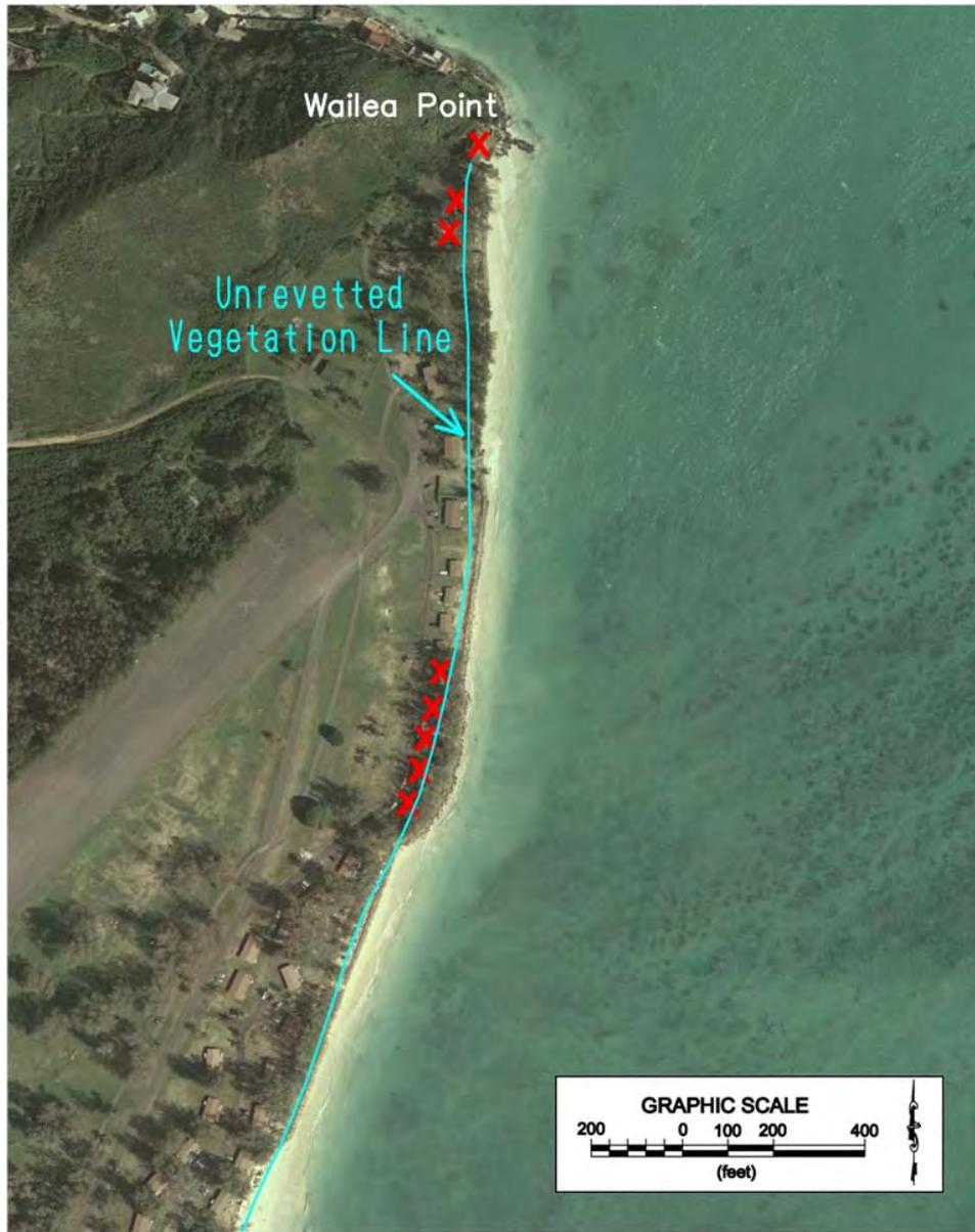
**Figure 36 Shoreline response to removed revetments—Bellows AFS**
